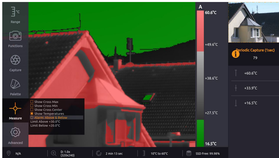
Figure 13.7: Alarm display – ABOVE & BELOW.
