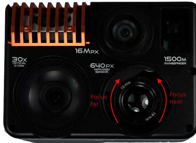
Figure 7.9 – Short distance - rotate the lens counter-clockwise. Long distance - rotate the lens clockwise
