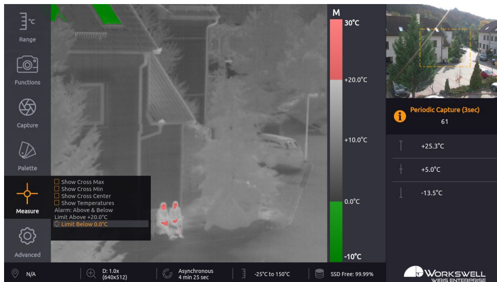
Figure 13.7 – Alarm display – ABOVE & BELOW.
