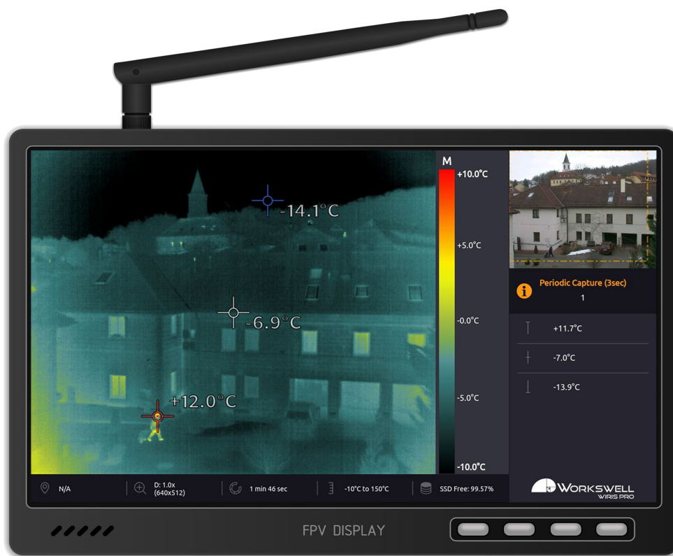
Figure 6.1 – Workswell WIRIS Enterprise connected to a standard FPV monitor (monitor not included)
