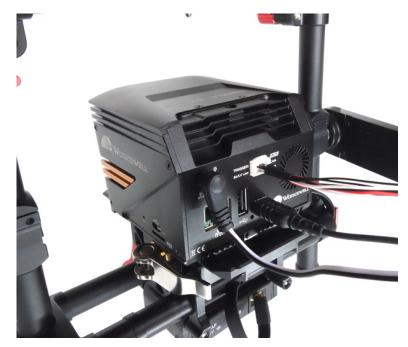
Figure 10.1: WIRIS Pro - DJI Ronin connection.
