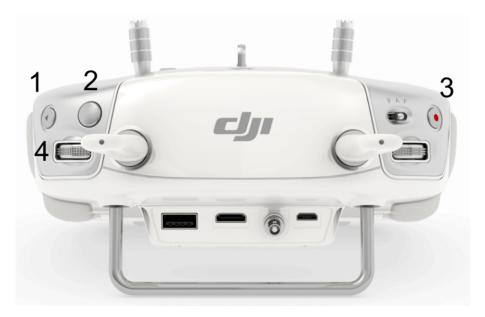
Figure 10.2: DJI Lightbridge 2 controller.
