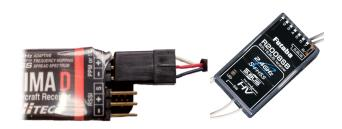
Figure 8.4: Example of connecting SBUS to OPTIMA D receiver.
