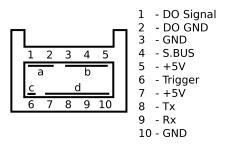
Figure 11.1: Connector pinout with Digital Outputs configuration.
