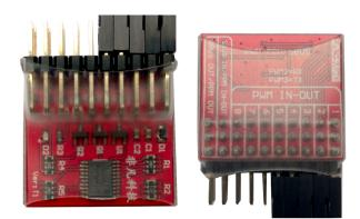
Figure 8.2: OEM PWM converter
