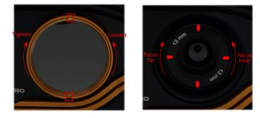
Figure 7.9: Short distance - rotate the lens counter-clockwise. Long distance - rotate the lens clockwise
